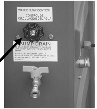
Open water flow valve 1 1/4 turns to allow water to fill reservoir.
